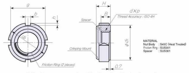
\* Simultaneous processing of the thread and the bearing surface.
