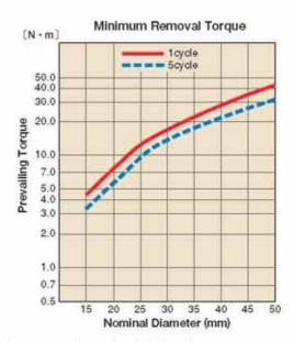
The prevailing torque is generated by the reaction to the spring acting on the shaft threads. (The graphs can be used for reference when using lubricated fasteners.)
