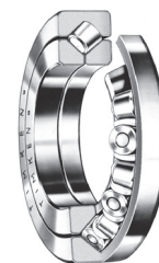
Fig. 106. TXR crossed roller bearing.
