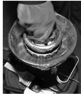
Fig. 16. Mechanical grease packer.
