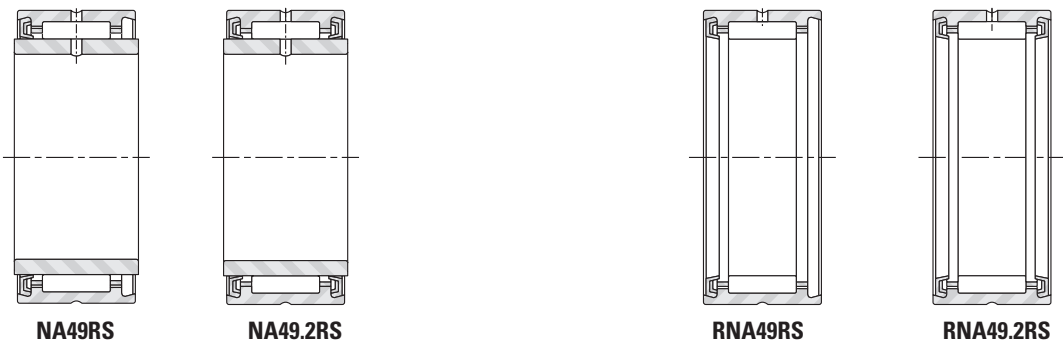
Fig. B4-3. Sealed needle roller bearings with inner rings
