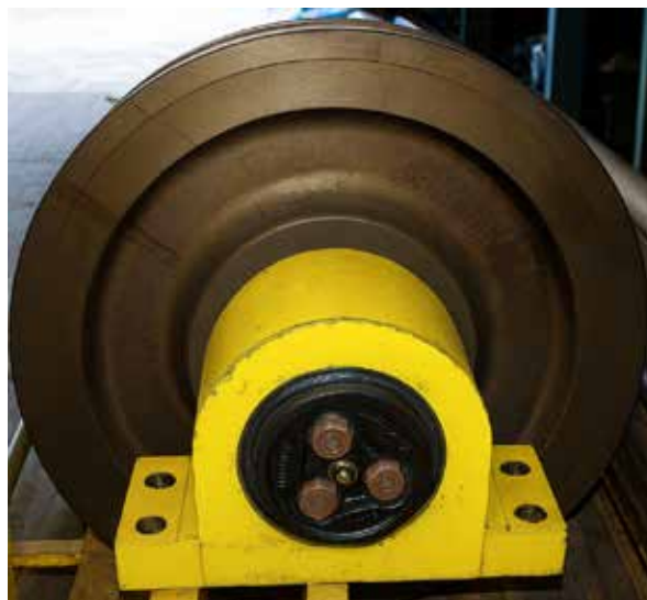
Fig. 12 AP bearings used in pillow block application
