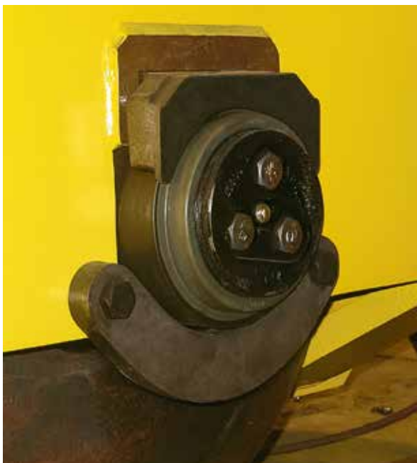
Fig. 8 Narrow adapter mounting on trolley safety bar
