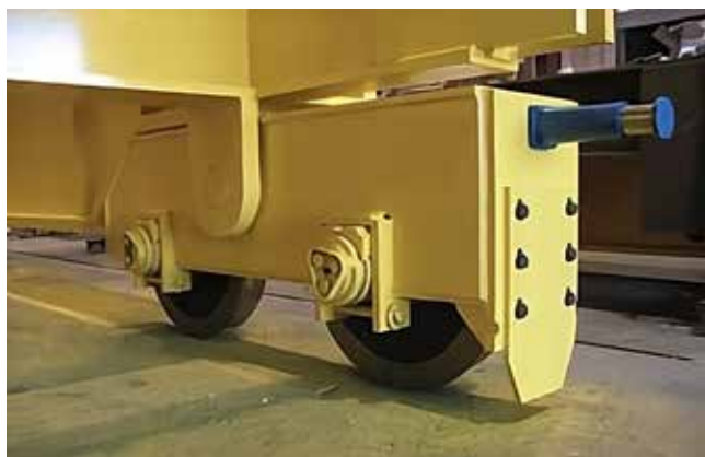
Fig. 5 Standard end cap design
