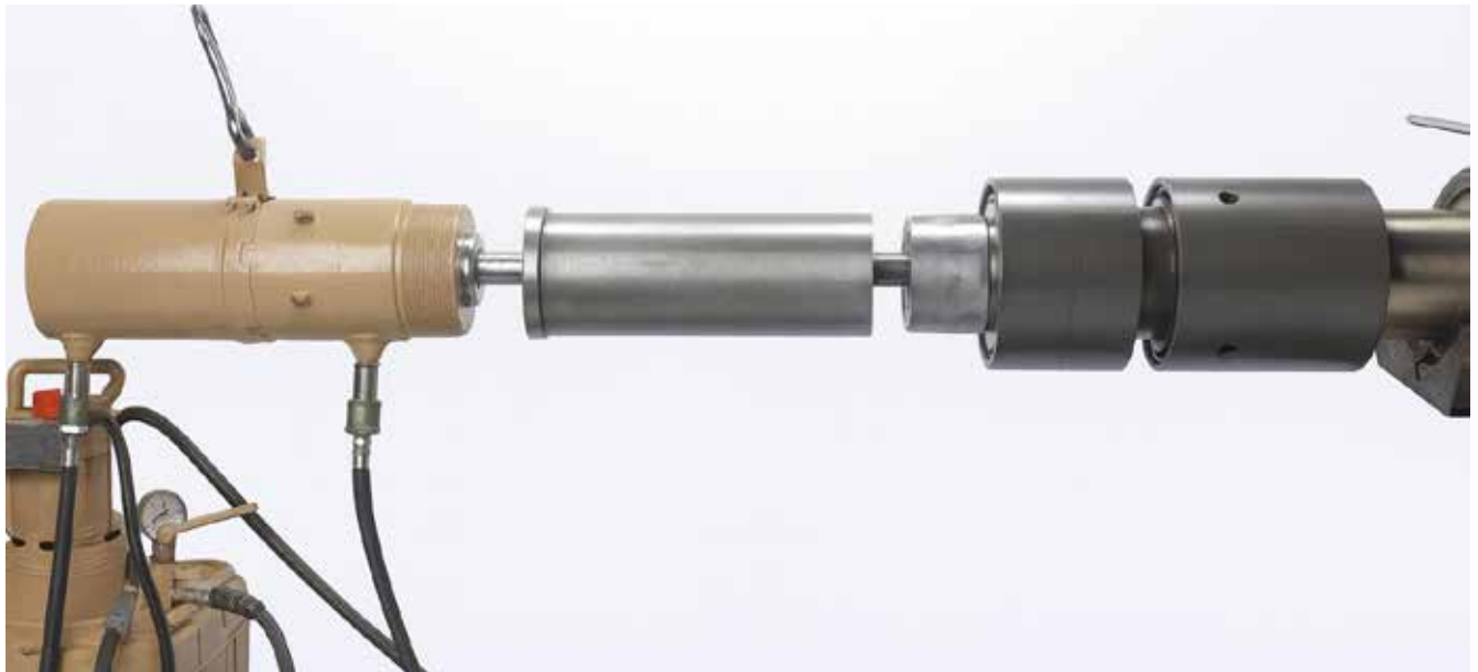
Fig. 28 Tooling used to push bearing onto shaft
