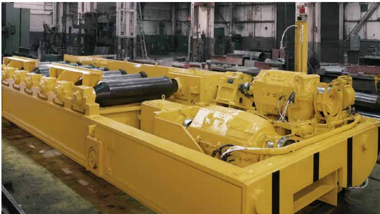
Fig. 10 A standard narrow adapter is used at both positions to ensure positive radial location of the AP bearing cups. A close clearance is provided between thrust lugs and the sides of the adapters to keep axial movement of the roll to a minimum.
