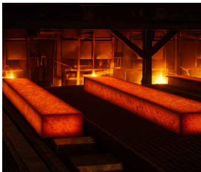
Fig. 11 AP bearing equipped runout tables
