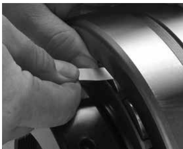
Fig. E-7. Measure RIC before installation.
