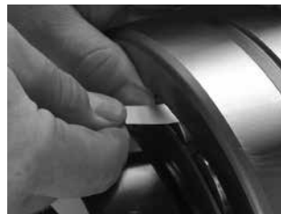
Fig. E-3. Measure RIC before installation.
