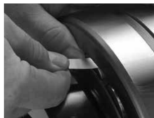
Fig. D-3. Measure RIC before installation.
