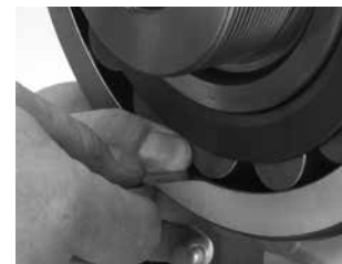
Fig. D-4. During mounting, the RIC should be checked at the unloaded roller.
