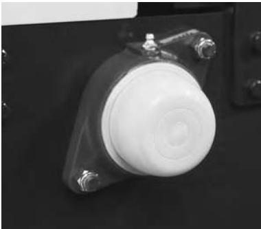
Fig. A-29. Safety end caps protect against rotating stub shafts.
