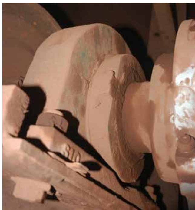
Fig. 20. Timken Mounted Split Cylindrical Roller Bearing is shown here in a steel industry application.
