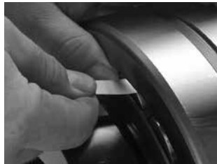
Fig. 91. Measure RIC before installation.
