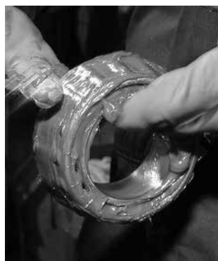
Fig. 149. Grease can easily be packed by hand.
