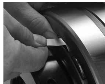
Fig. 95. Measure RIC before installation.
