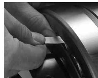
Fig. 97. Measure of RIC before installation.
