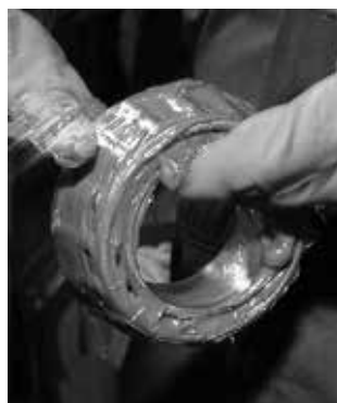
Fig. 23. Grease can easily be packed by hand.
